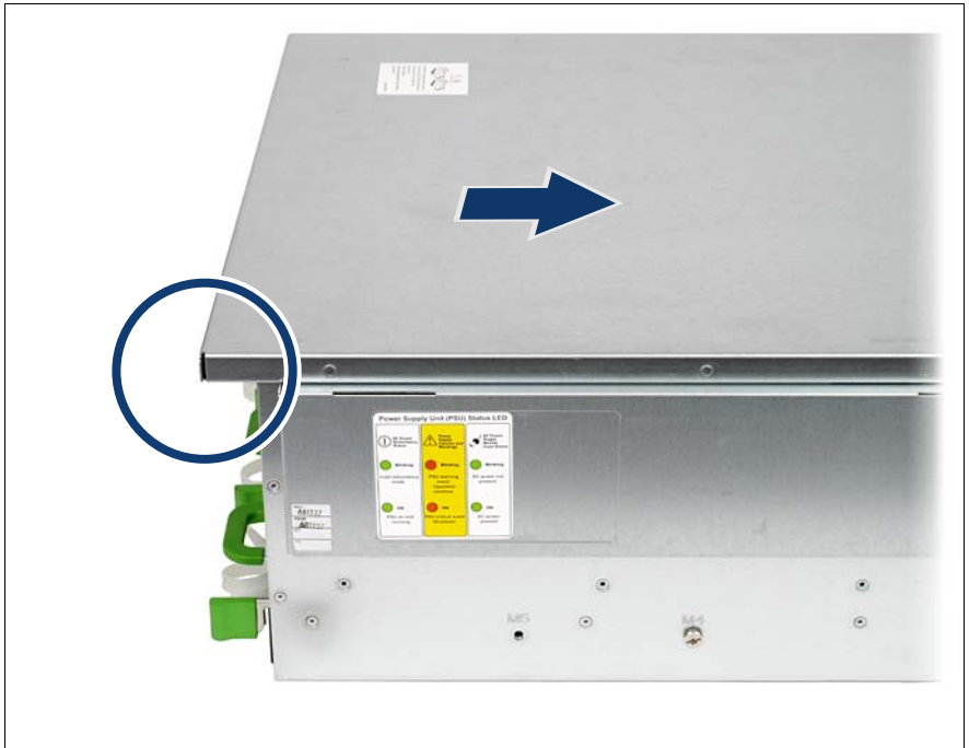
Figure 45: Placing the housing cover
